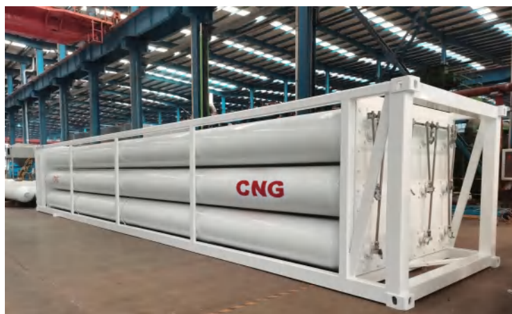
CNG Tube Trailer
